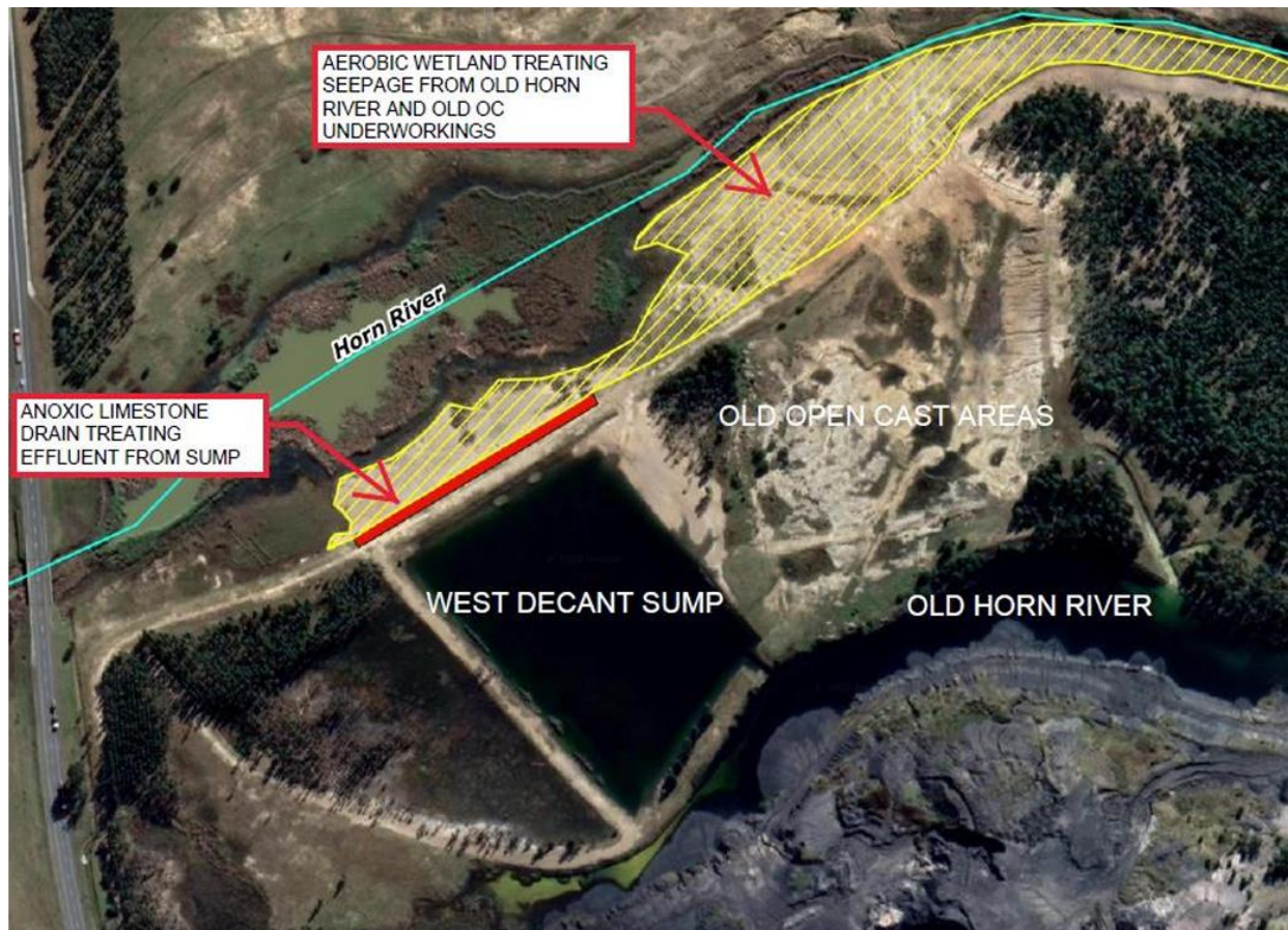
Figure 1-3: West Decant Sump area to be treated with ALD and cut off Aerobic Wetland along Horn River boundary
